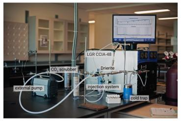
The new MDRU Mineral Isotope Analyzer is based on Off-Axis Integrated Cavity Output Spectroscopy (OA-ICOS), characterized by relatively low initial capital cost, low maintenance, and inexpensive consumable requirements. The off-axis laser alignment is particularly robust, introducing the potential for field or mine site deployment.
