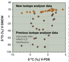
The new analyzer's greatest advantage compared to MDRU's former stable isotope analyzer is the ability to analyze sulfide-bearing carbonate samples and pulps which was previously impossible because of interference of H<sub>2</sub>S and CO<sub>2</sub> during laser absorption. This now allows detection of isotope ratios in ores, mineralized rocks, and host rocks containing diagenetic pyrite.
