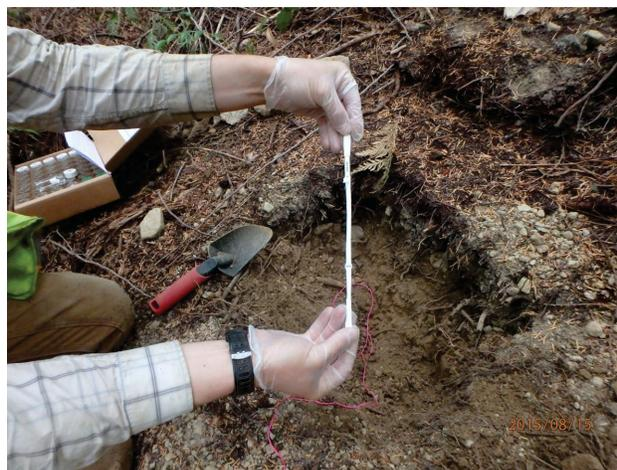
**Figure 2.** An AGI Gore Module activated-charcoal organic-compound collector being retrieved after two months (Image: M. Bodner).
